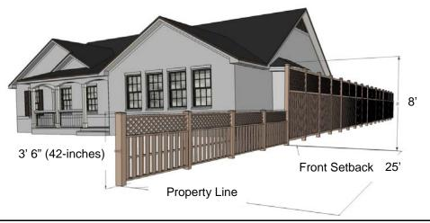
If placing a fence on a retaining wall or raised bed, the total height will be measured from grade level as determined below.
